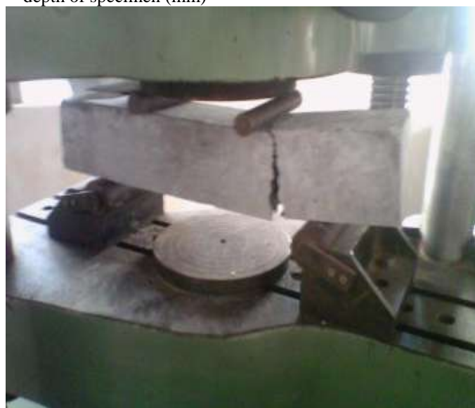
Fig.4. Testing the flexural strength of specimen
