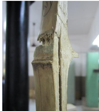
Figure 5 Failure of bamboo strip (node split)
