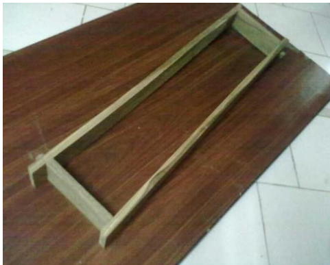
Figure 7 Mould of size (in to in) 900 mm x 250 mm x 75 mm
