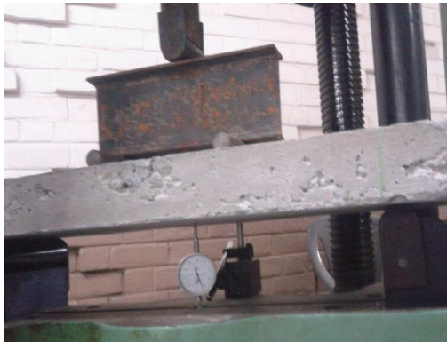
Figure 14 Flexural test setup of slab panel
