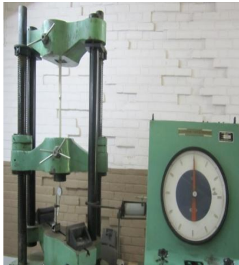
Figure 4 Set up of tensile strength of bamboo strip.
