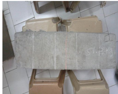
Figure 8 Plain concrete slab panel
