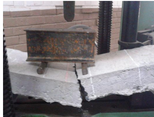
Figure 15 Brittle failure of slab panel
