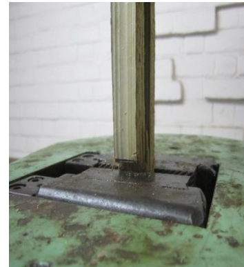
Figure 6 Failure of bamboo strip (end split)
