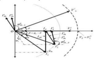
Fig. 7. Current-based phasor representation of the proposed UPQC-S approach under voltage sag condition.
