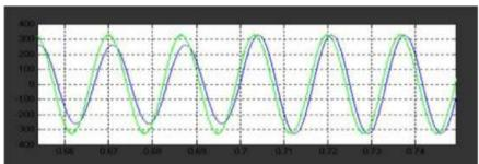
(j) Enlarged power angle  $\delta$  during voltage swell condition. Fig. 6.2. Simulation results: active and reactive
