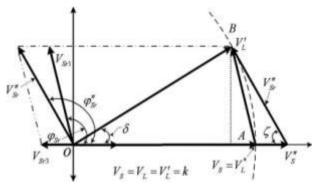
**Fig 9**. Phasor representation of the proposed UPQC-S approach under voltage Swell condition. For voltage swell compensation using active power control approach
