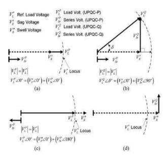
**Fig. 4** Voltage sag and swell compensation using UPQC-P and UPQC-Q: phasor representation. (a) Voltage Sag (UPQC-P). (b) Voltage Sag (UPQC-Q). (c) Voltage Swell (UPQC-P). (d) Voltage Swell (UPQC-Q).
