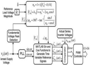
Fig. 11 Reference voltage signal generation for the series inverter of the Proposed UPQC-S approach.
