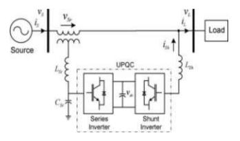
Fig.1. Unified power quality conditioner (UPQC) system configuration.
