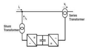
Fig.2.Principle configuration of an UPFC
