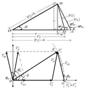
Fig.5 Phasor representation of the proposed UPQC-S approach under voltage sag condition.
