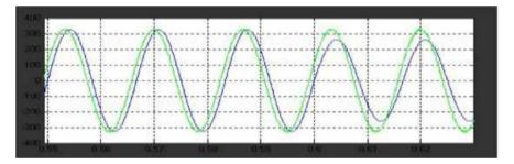
(h) Shunt inverter injected current
