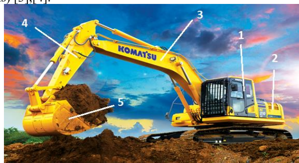
Fig. 5. 1. Cabin, 2. Engine, 3. Boom, 4. Stick, 5. Bucket
