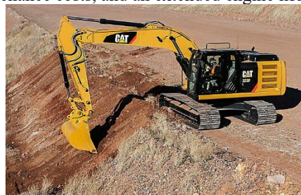
Fig. 8. Hydraulic excavator-backhoe from the manufacturer Caterpillar, model CAT 323F LN
